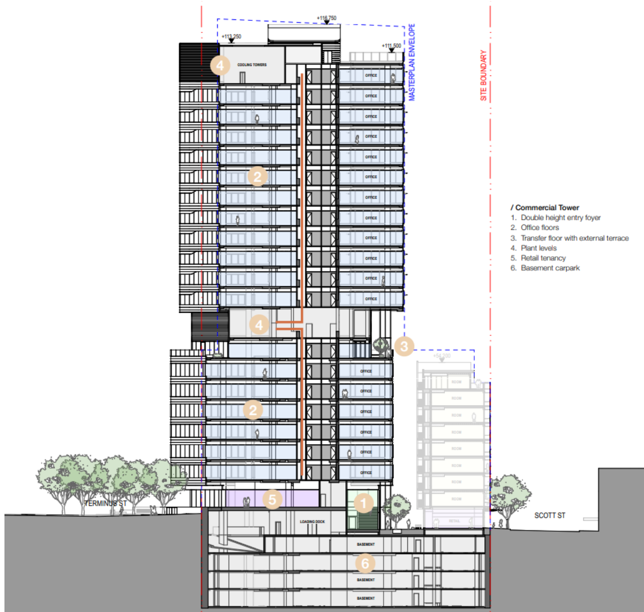
Figure 36 Commercial office building level by level use (north-south section)
